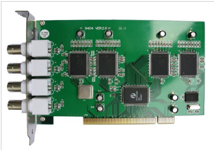
Multichannel capture card, Philips Saa7130 chipset
